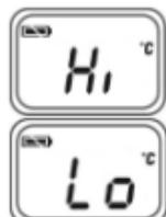
'Hi' or 'Lo' is displayed when the temperature being measured is outside of the range of the instrument, 'Hi' when higher than +220°C (428°F) and 'Lo' when lower than -33°C (-27°F).
